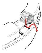
Patented Air Flow Control technology delivers optimal passive attenuation across all frequencies, without increasing earcup size or weight. A patented baseplate chamber and high-tech non-woven layer manage the flow of air inside the earmuff to control how sound reaches the ear. The result is better, more consistent overall attenuation for virtually all industrial noise environments.
